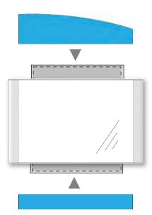
1/8" Thick Acrylic or Wood Laminate Accent Shape Attaches to the Aluminum Connector, Flush with the Top (and/or Bottom) of the Arris Frame.
